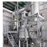
PulsReg®-Zentral Pulsed regenerative burner system
