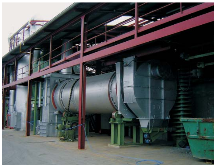
Fig. 2: Rotary drum of the drying swarf plant
